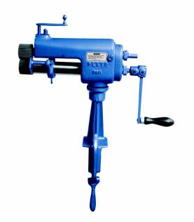
A combination Rotary Machine embodying all the features of the Throatless Machine with the added features of a 7" throat, and arbors designed to utilize crimping, beading, furnace collar edging and offset rolls. See Roll Chart for rolls available.
