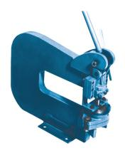
These deep throat hand punches are actuated by an eccentric cam rolling on a heavy duty bearing. Ram is held securely by the gibs. Die shoe is removable and adjustable, permitting the use of close fitting punches and dies. 3/16" adjustment in ram position is provided.
