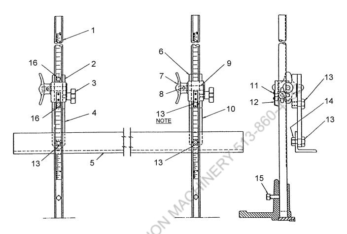
NOTE: R.H. LINK (10) IS ASSEMBLED TO R.H. GAUGE HOLDER (6) WITH ONE PIVOT STUD (13) TO PROVIDE FOR ANGULAR SETTING OF BACKGAUGE.
