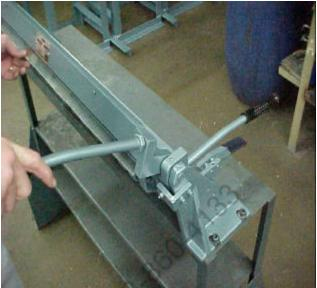
Return the bending lever to its original position at the rear of the machine. Place the partially formed 5. part against the nose of the bending blade. Pull the bending beam lever toward you while holding the work material in the machine until the blade contacts the part. Push the lever down to finish forming the flange.
