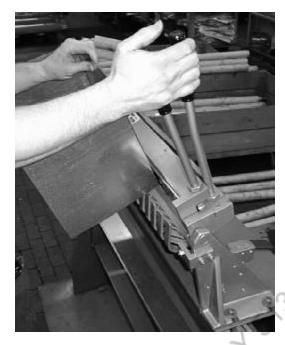
While you hold onto the work piece, return both of the beam levers to their starting position. 5. Allow the work piece to rotate with the beams while supporting it with your free hand. The ane le duct will slide free of the bending blade as the levers approach vertical.
