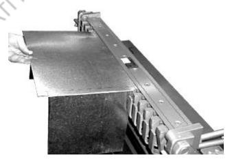
2. Make sure that the work piece is inserted under the bending blade as far as it will go. Pull the bending beam lever toward you until it stops.
