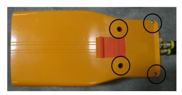
Remove the 4 Phillips screws from the foot pedal body and remove the cover.
