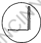
1 1/4" Standing Seam With Right Angle Flange Up to 1 1/2" available Both standing seam and right angle flange are formed with same roll set
