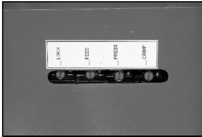
Figure 4-3 Air Valve Station
