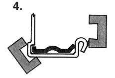
Open jaws halfway, roll tool towards inside of the duct to hook jaw on inside of the groove. Opposite jaw's back leg should line up with the hem on the outside of the T.D.C. flange.
