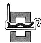
Squeeze tool handles together until the corner snaps into the groove on the back side of the T.D.C. flange.
