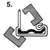
Squeeze tool handle to bend hem over in order to hold corner in place.
