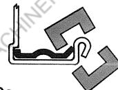
Note: When the corner is in place, squeeze the angle side again to set it down as far as possible. This procedure makes it easier to fold the hem over.
