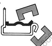
With the front teeth (legs), grab the corner near the hem lip on the angle edge and the other jaw will line up on the T.D.C. flange near the end.
