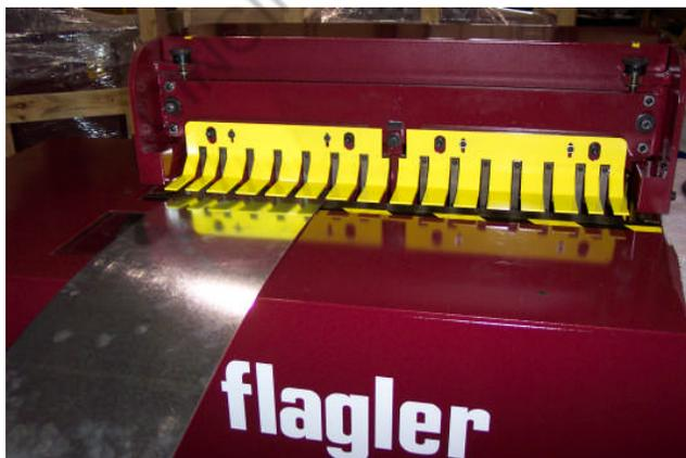
The left side of the machine is where the clamping motor is connected to thus it is the stronger side of the machine.
