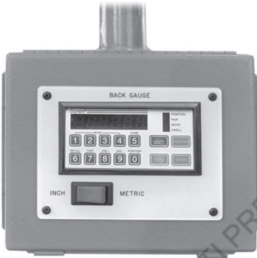
Power Front Reading Backgauge Adjustment w/5 Station NC "GO-TO" Positioner on Pendant
